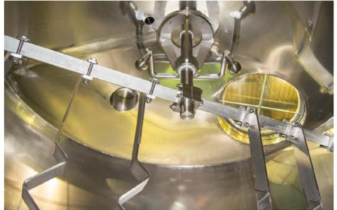
Interior of the Lauter tun with system of nozzles for wort rinsing and CIP spray balls.
