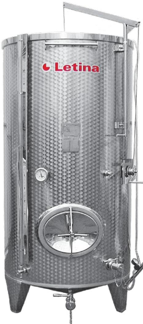
**VARIABLE CAPACITY TANK** Thanks to the floating lid, you don't have to fill the variable capacity tank to its brim. The inflatable gasket achieves an airtight seal, preventing oxygen contamination. Moving the floating lid into place and securing the air seal is easy with the lifting arm and hand pump.
