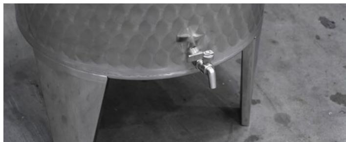
**MIXING TANK** The built-in flow breaker helps the agitator efficiently mix, agitate or gently stir your products. A folding cover comes standard with the mixing tank to make charging easy.
