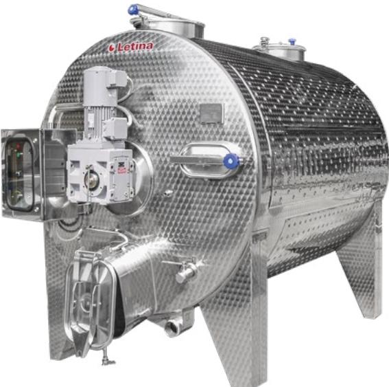
**HORIZONTAL FERMENTER** The horizontal fermenter was designed to perfect the maceration of white wine, vinification of red wine and fermentation of spirits or liquors. A geared motor powers an agitator spanning the length of the tank. The motor is equipped with an inverter, allowing an adjustable speed in either direction.
