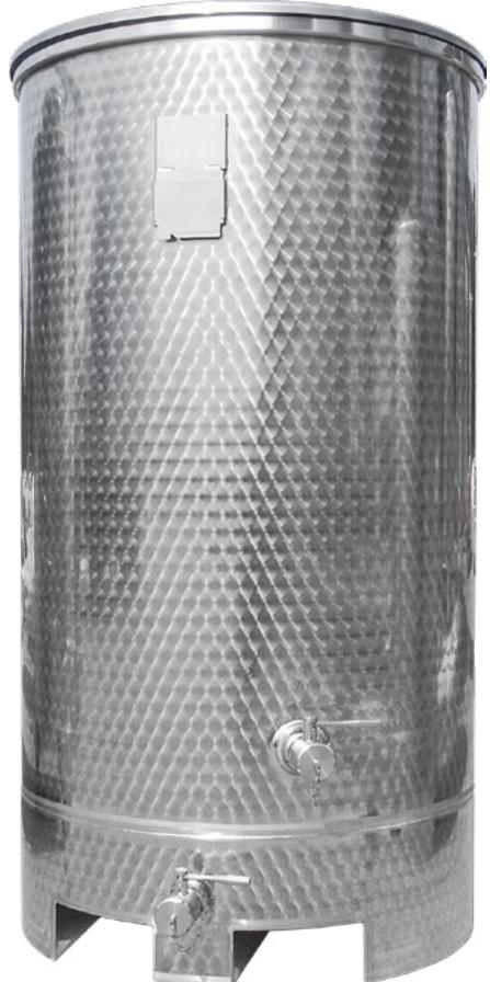
**FORKLIFT TRANSPORT TANK** The forklift transport tank is a vessel designed to be easily maneuverable with a forklift. It has a sturdy skirt with 2 slots for the lifting forks. Usually it is a variable capacity tank with a floating, air-sealed lid, and an optional lifting arm.
