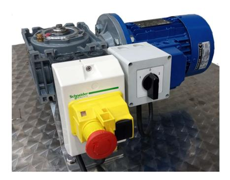
In the picture is seen a motor protection switch and 1-0-2 switch. The switch 1-0-2 is used to change the direction of rotation.
